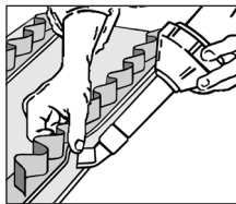
Profile with base for welding by hand with the Leister or using our LSM 1200R machine.
