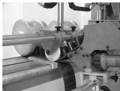
Profile with base for welding by hand with the Leister or using our LSM 1200R machine.
